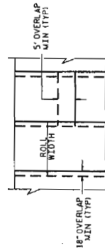
GEOTEXTILE FOR ROCK EMBANKMENT OVERLAP DETAIL (PLAN VIEW)
